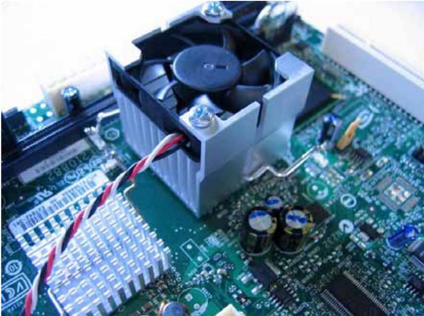
Therefore press down the metal holding clamp and then rotate the heatsink carefully.
