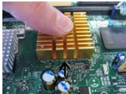
Now insert one tail of the metal holding clamp on the mainboard (arrow 1 on the picture), hold it down with one finger and then insert the other tail on the mainboard (arrow 2 on the picture).
