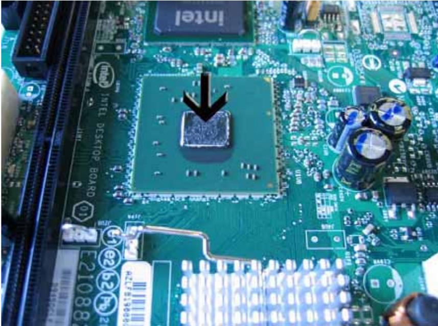
Remove the protection foil from the new heatsink and place it with soft pressure on the chipset. Take care of positioning in a way so you can insert the metal holding clamp later on (see pictures below)
