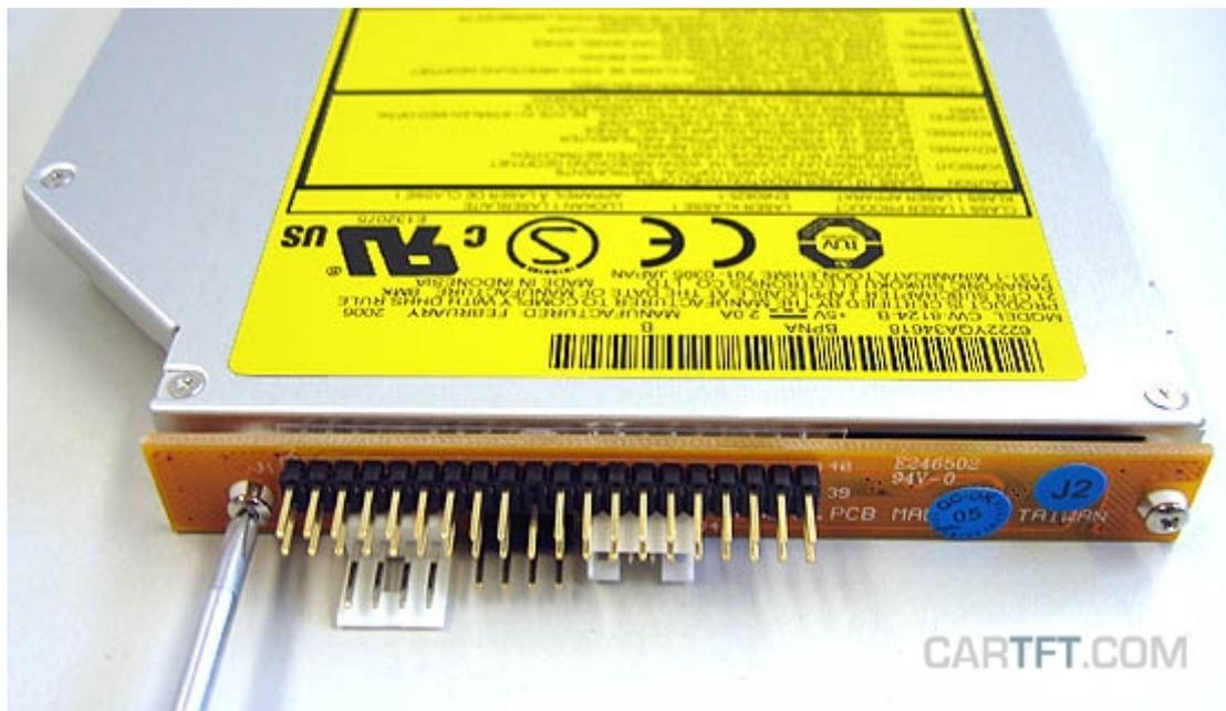
Then the CD/DVD drive gets installed at the drive mounting unit, which gets screwed at the side with 2 small screws:
