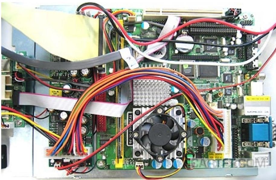
The ATX-cable should be laid like shown in the picture:
