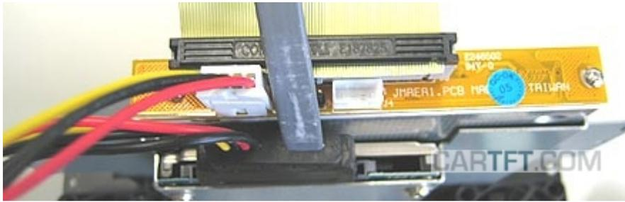
The ATX cable is attached so that the end is put with the further power connections on the M1-ATX power supply and the other one end on the motherboard. The ATX cable or all other cables, too, have to be laid flat, compact and space-saving, so that the floor metal can be put into the VoomPC-2 enclosure without problems. This is what it should look like:
