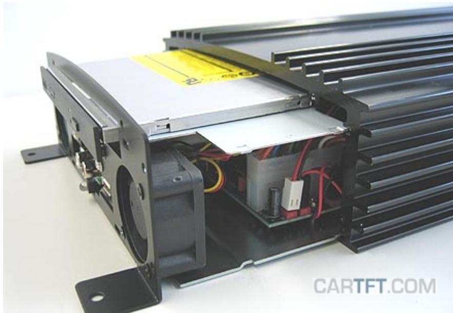
After that the 6 case screws have to be tightened.
