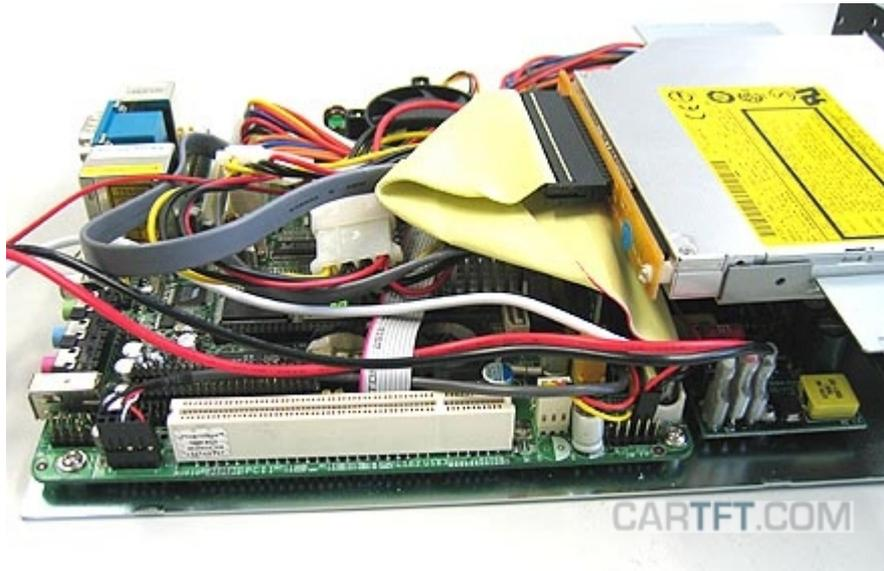
The floor metal gets pushed with the drive mounting unit into the enclosure carefully, so that no cable gets stuck or gets damaged.
